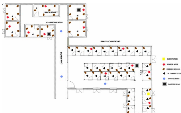
Fig. 1: Deployment Scheme of RSSI Sensor
